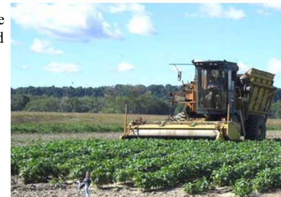
FWA's bean harvester scoops up the beans, blows out the vines and stalks and throws the beans up into the hopper.
