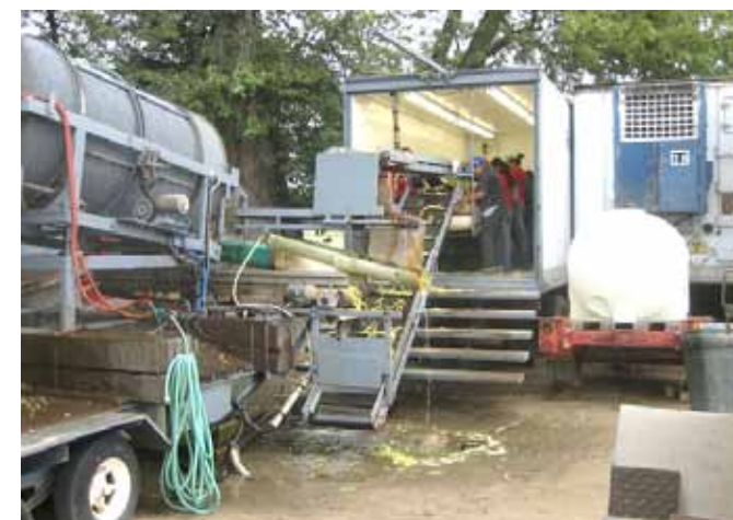
The freshly picked beans go from the harvester into the washer, then into the dryer, up the conveyor to the packing table where workers fill the boxes for delivery to the regional market or directly to supermarkets. In past years 600 acres of beans yielded $2 million pounds of beans.
